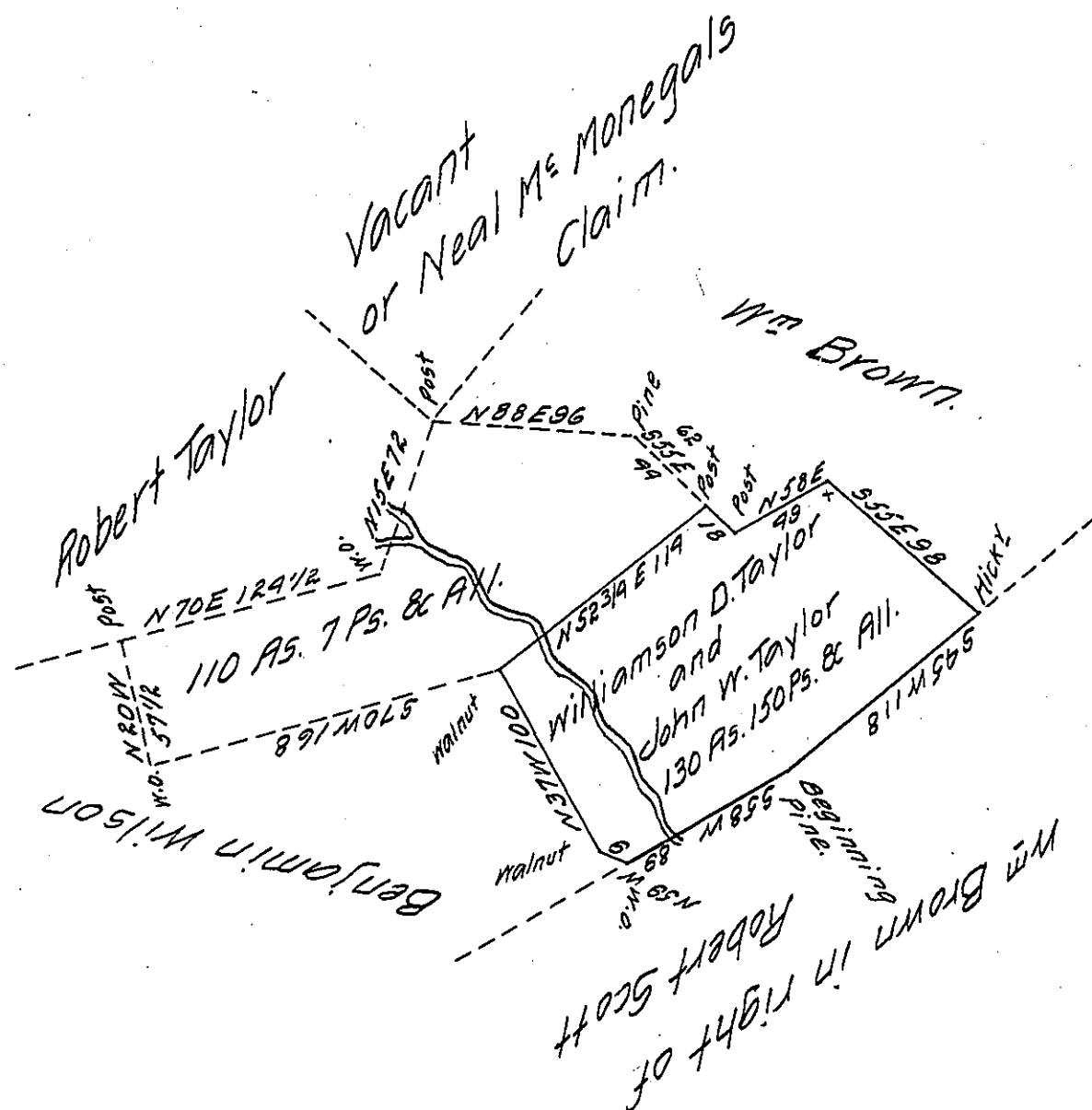
Draft of a part of a tract of land copied and constructed from a Draft of a survey made in the name of John Templeton, surveyed the 23d June 1767, on Application No 1988 granted to John Templeton dated the 27<sup>th</sup> day of Novr 1766, containing in the whole 240 acres and 157 Perches and usual allowance.
